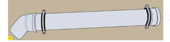
After the pipe and fittings are jointed, place them and tighten the clamps.
