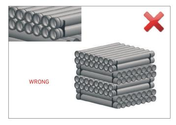
Pipes and fittings with socket are placed in a way that they will not stay on top of each other.
