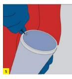
Remove the burrs on the external edges with a knife or scraper.
