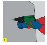
Drill the marked points with a driller and place dowels into the holes.
