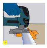
Cut in 90° angle by using a coping saw or a proper cutter.
