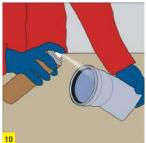
Apply a lubricating liquid (silicone etc.) to the socket part of the pipe.
