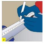
When interval measurements are required, mark the pipe with the desired measurements.
