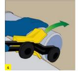
Chamfer the spigot of pipe by using a chamfering device or thick riffler.
