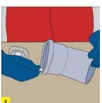
Mark the part of the pipe that will be attached to the fitting as much as the jointing distance.
